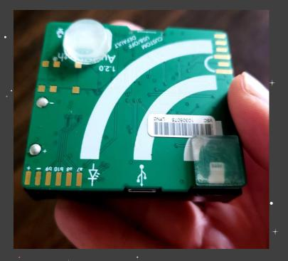
AudioMoth is a low-cost, full-spectrum acoustic logger, based on the Gecko processor range from Silicon Labs. Just like its namesake the moth, AudioMoth can listen at audible frequencies, well into ultrasonic frequencies. It is capable of recording uncompressed audio to microSD card at rates from 8,000 to 384,000 samples per second. Open Acoustic Devices
